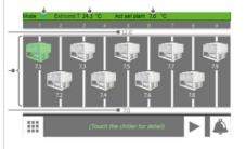
Each module has its own electrical panel guaranteeing continuity even if one module malfunctions Multichiller Evo controller can manage upto 9 units in parallel mode
